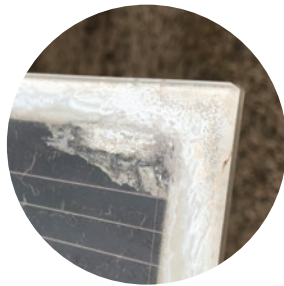
Delamination 9 years SW USA
