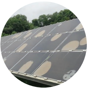
Glass/encapsulant delamination 8 years West India
