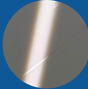
Widespread backsheet cracking PVDF
